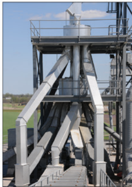
Modified Rapat distributor with enlarged spouting (middle platform) below a second, new Rapat distributor (top platform). Photo by Tucker Scharfenberg.
