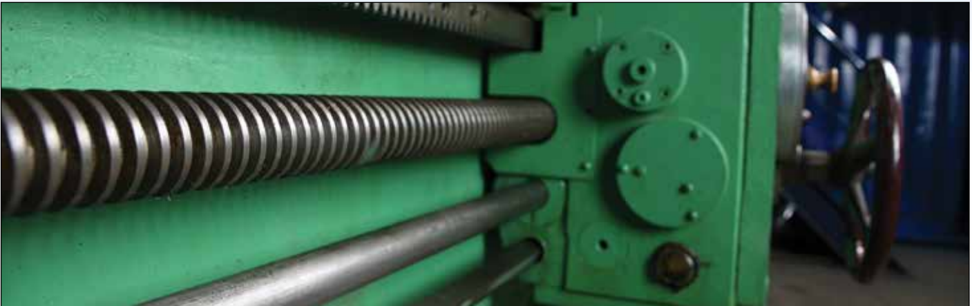
Nook/Thomson acme screw used in a manual lathe
