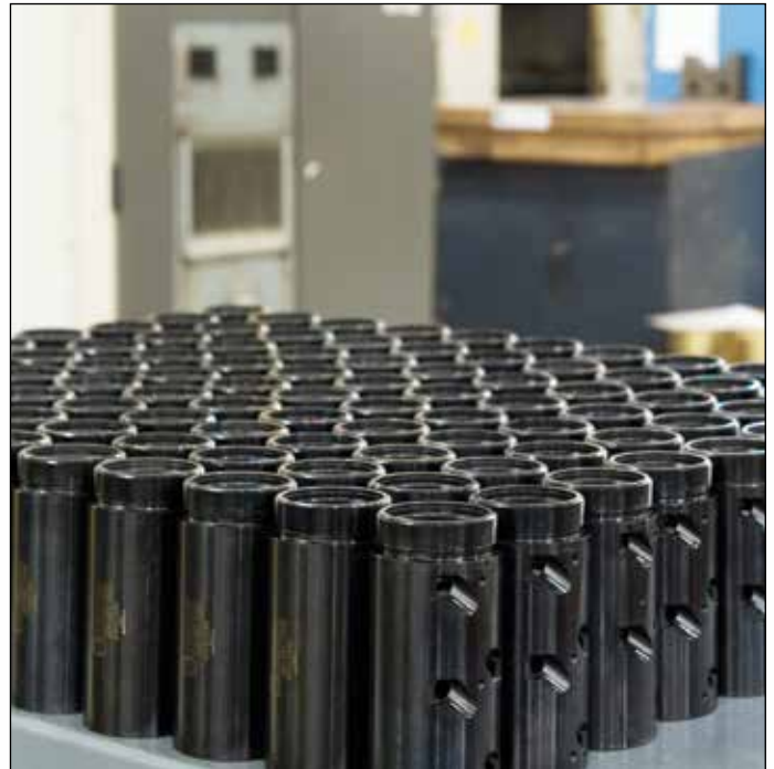
Nook/Thomson 2.00" diameter ball nuts
