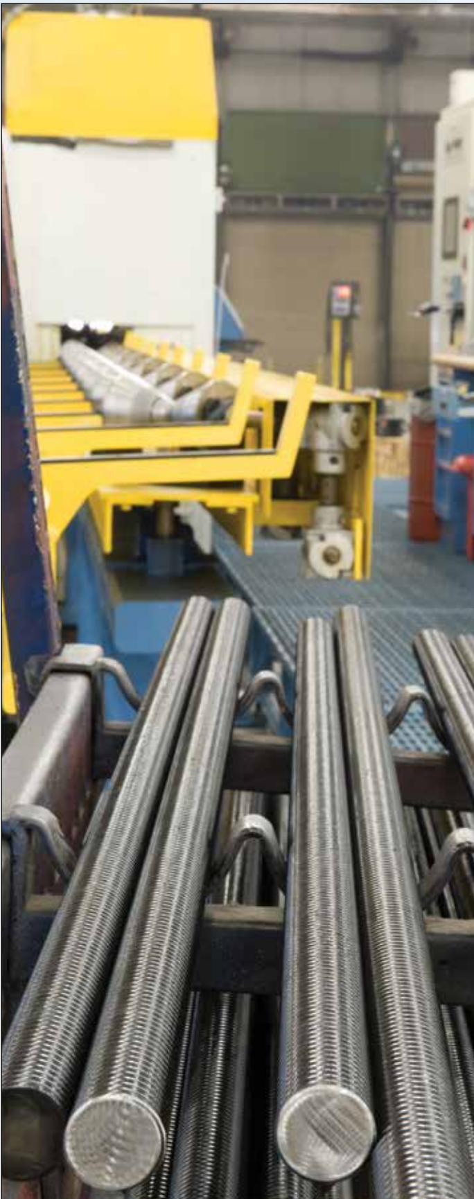
Precision heat-treatment of ball screws
