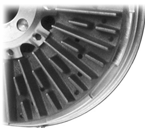
Cross-drilled rotor with heat dissipating fins.
