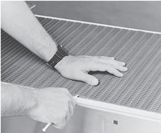
Figure 1: Plastic modules joined by hinge rods
