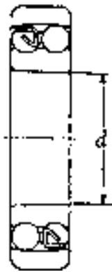
Tapered Bore 12K Taper 1:12
